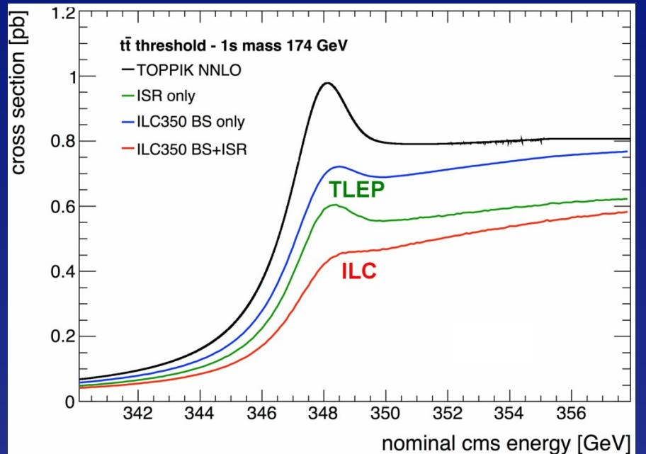
Beamstrahlung @TLEP is important for machine design but benign for physics:
