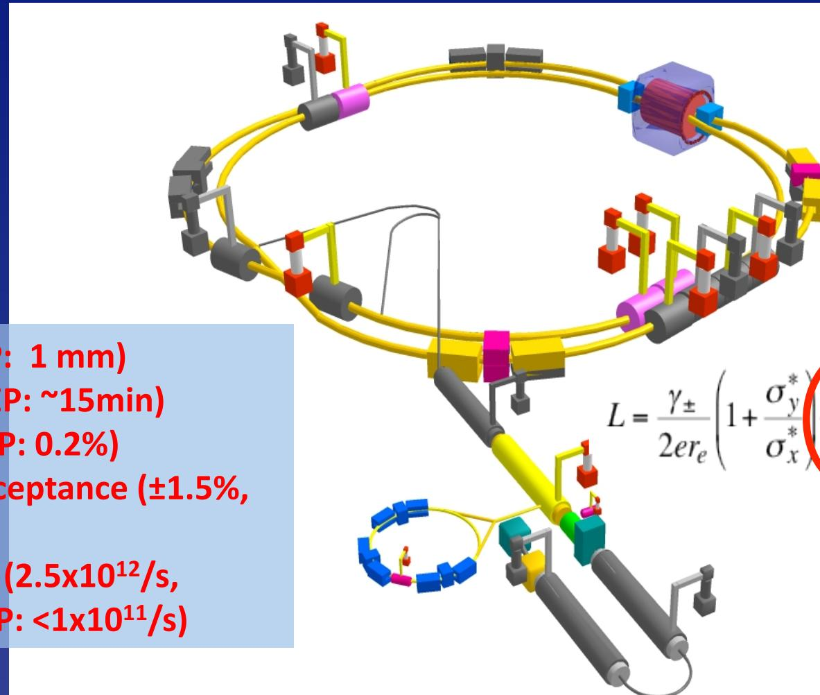
$$L = \frac{\gamma_{\pm}}{2er_e} \left( 1 + \frac{\sigma_y^*}{\sigma_x^*} \frac{I_{\pm} \xi_{\pm y}}{\beta_y^*} \frac{R_L}{R_y} \right)$$
