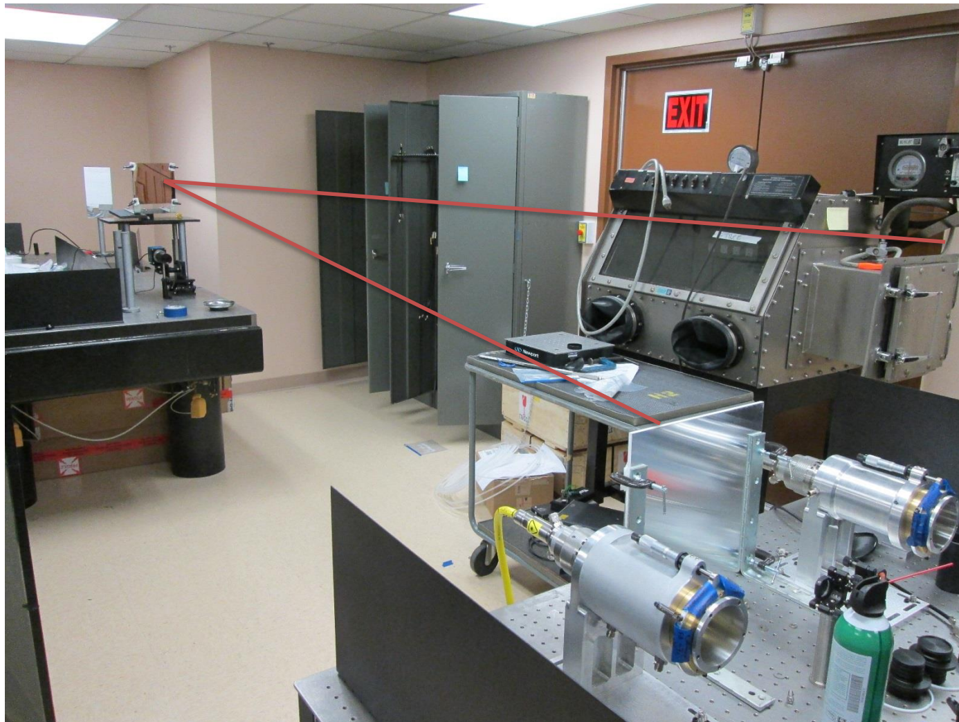
One setup showing a simulation of window reflection
