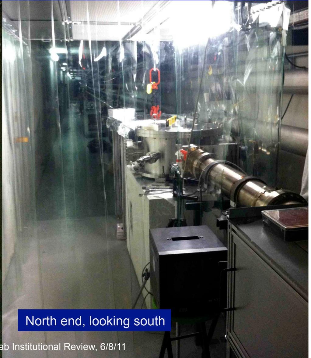
End station vacuum vessels hold custom optical cavity mirrors and eventually beamsplitters
