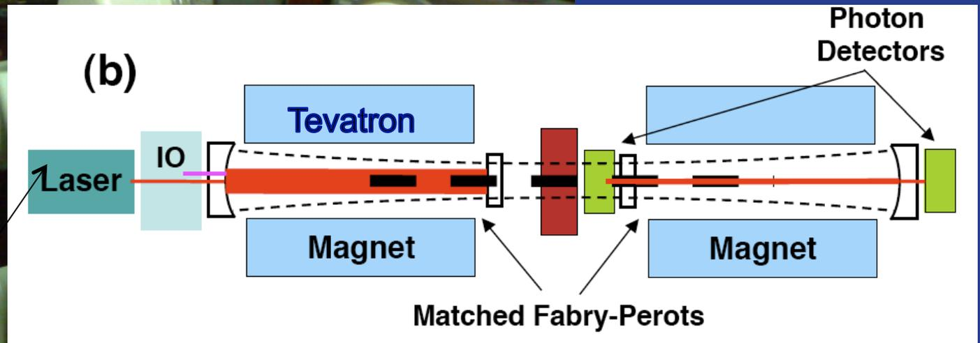
Increase photon flux from  $10^{19}$  to  $10^{24}$   $\gamma$ /s, increase L from 6 to 40m, resonantly detect
