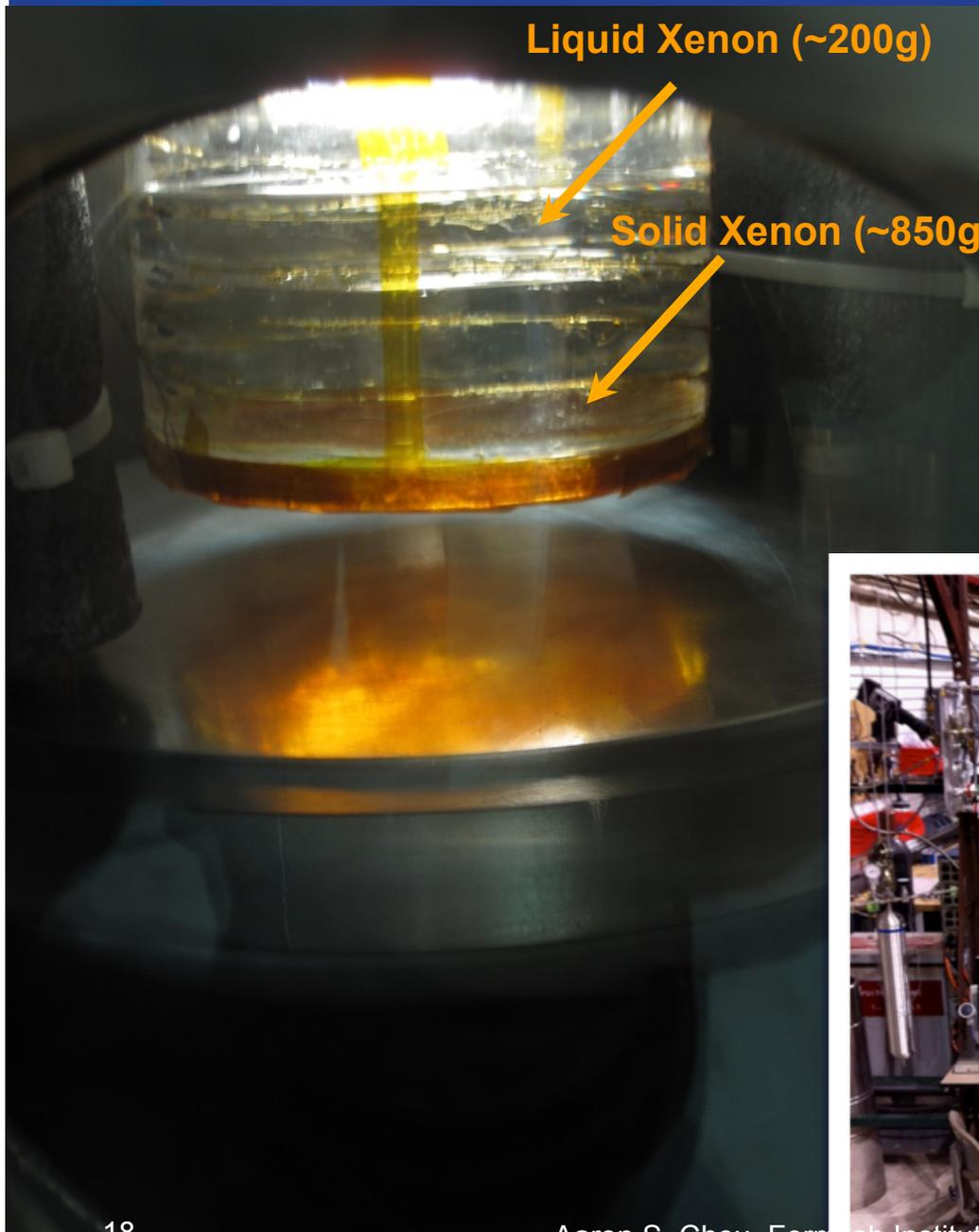
Phase-1: ~kg scale crystal clear solid xenon was successfully made (2010)
