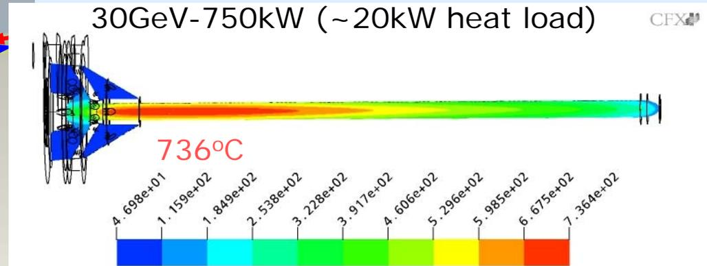
$\Delta T \sim 200K$   $\sim 7MPa$  (Tensile strength 37MPa)
