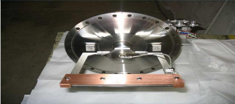
Oct.2015 New simplified primary assembly (just Al plate without any ceramic insulators):
