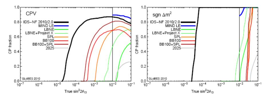
NOTE: For large  $\theta_{13}$  the LENF comfortably determines mass hierarchy for all CP phases ... so the (energy, baseline) optimization can be based just on CPV coverage.
