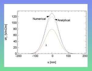
Vertical wake of one flange, assuming a Gaussian bunch with length  $\sigma_z=40$  mm (blue) and the analytical approximation (dashes). The bunch shape  $\lambda$  is also given in yellow (head to left).
