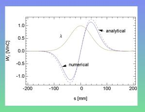
Longitudinal wake of one flange, assuming a Gaussian bunch with length  $\sigma_z=40$  mm (blue) and the analytical approximation (dashes). The bunch shape  $\lambda$  is also given in yellow (head to left).
