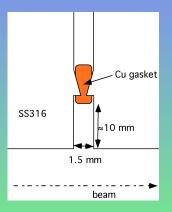
Flange geometry. The cross-section of the beam pipe is elliptical with half-heights  $a_x = 63$  mm,  $a_y = 32.5$  mm.
