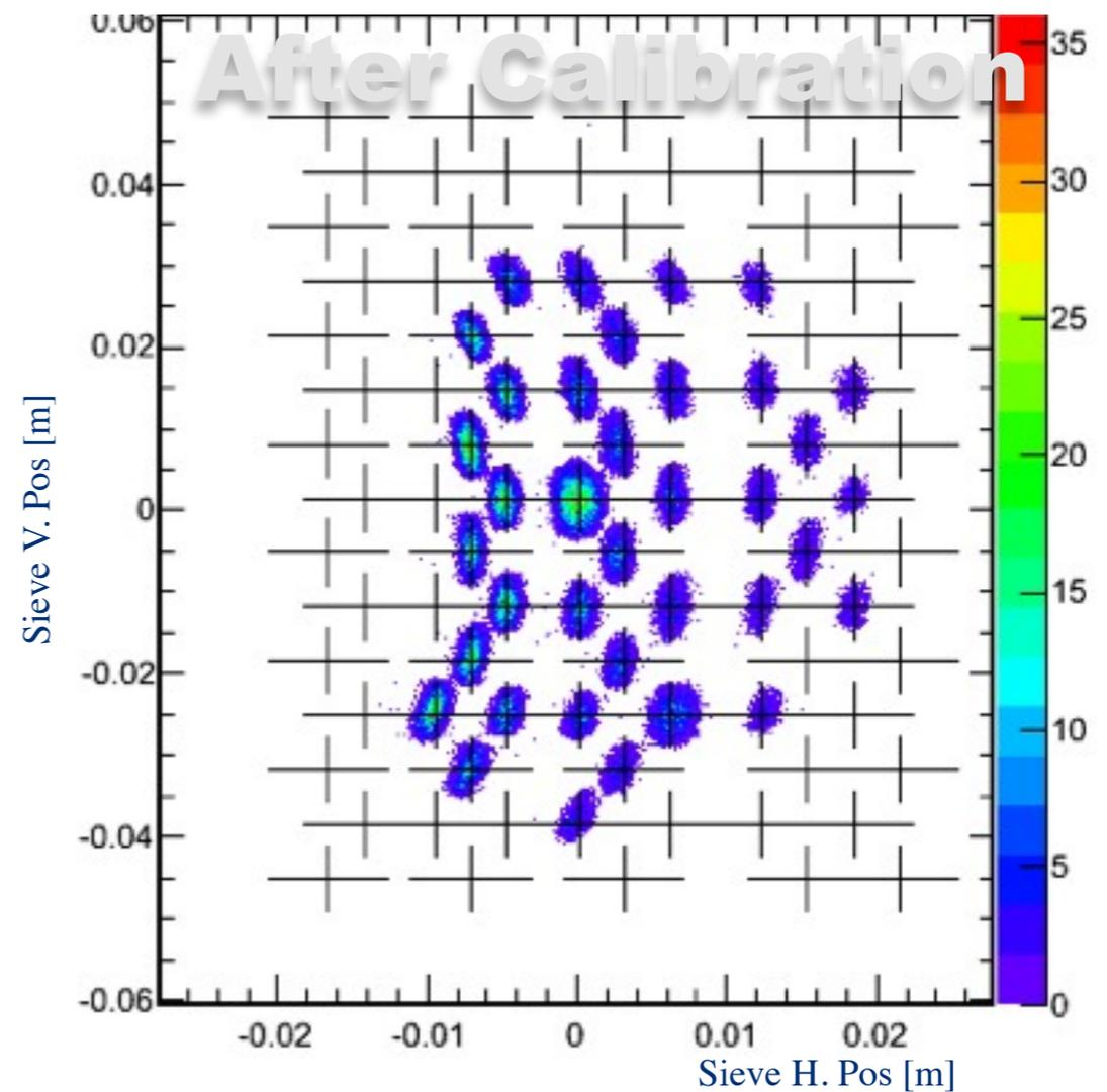
Left HRS calibration used 35 holes, Right HRS calibration used 38 holes
