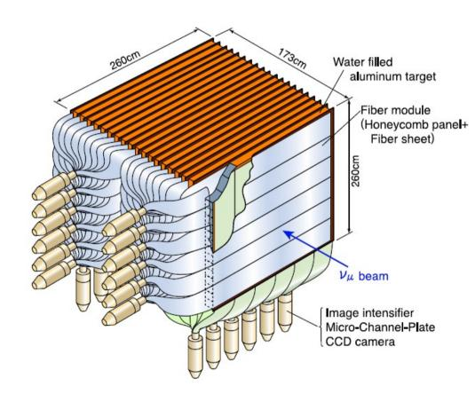
Design to improve the measurement of the neutrino energy and to study the neutrino interactions with high detection efficiency for low momentum particles
