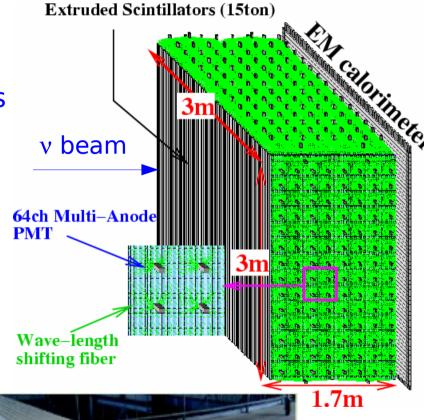
Its purpose is to distinguish electrons from muons by measuring the energy deposited
