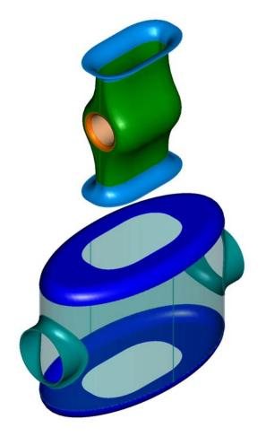
6 Welding steps required to fabricate the outer conductor
