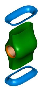
8 Welding steps required to fabricate the inner conductor
