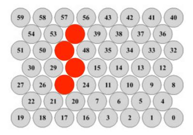
SLT: require 3 FLT within 20 µs for specified pixel patterns, noise rate 0.2Hz
