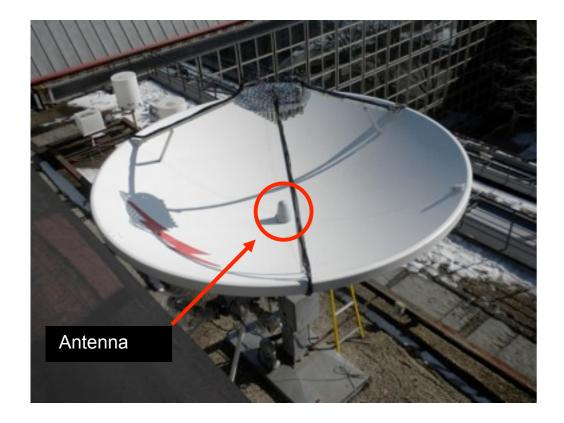
Log periodic antenna is directed at feeds sending 5 µs pulses
