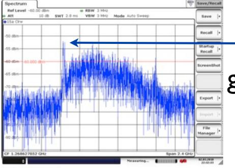
— Installed a IGHz band-pass filter, greatly reduced power in bursting lines
