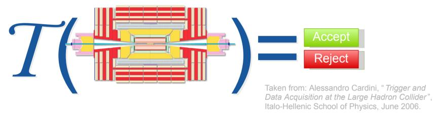
The *Data AcQuisition* (DAQ) system collects the data from the different parts of the detector, converts the data in a suitable format and saves it to permanent storage.
