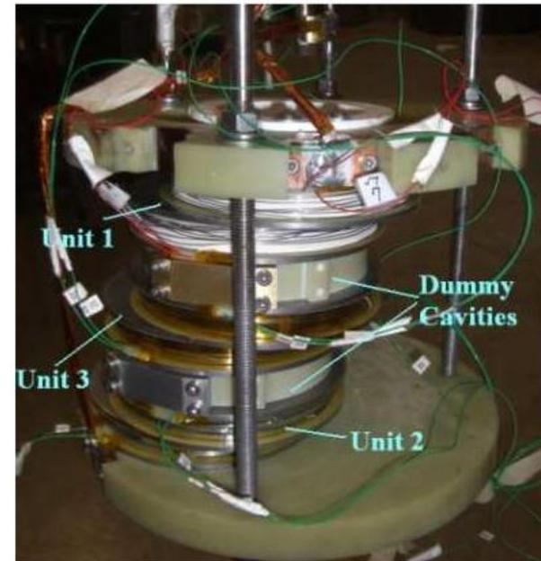
M. Yu et al. "Fabrication and test of short helical solenoid model based on ybco tape"
