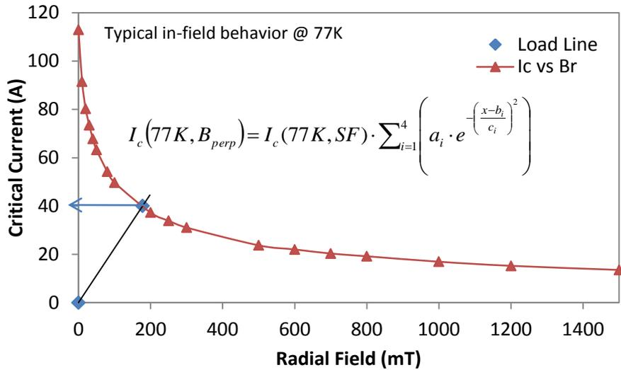
Expected coil current ranges were far below the nominal critical current measured on short samples due to self field impacting **perpendicularly** to the **ab** plane of the tape.
