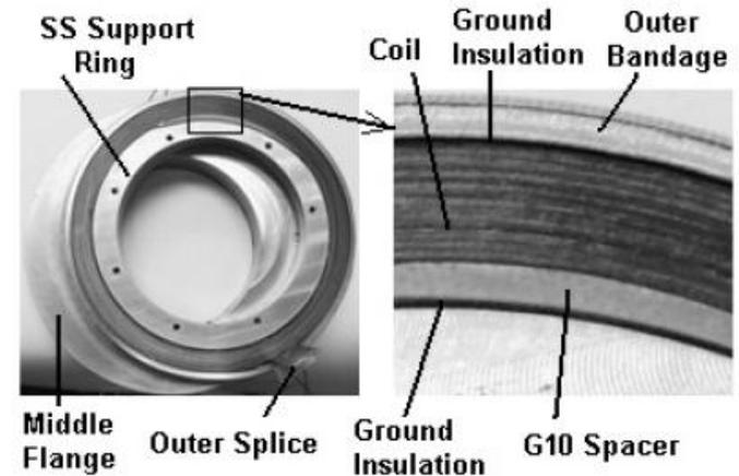
1. Coils assembled using commercially available 12mm wide SuperPower ybco tape. Dry Wound. Kapton insulation.
