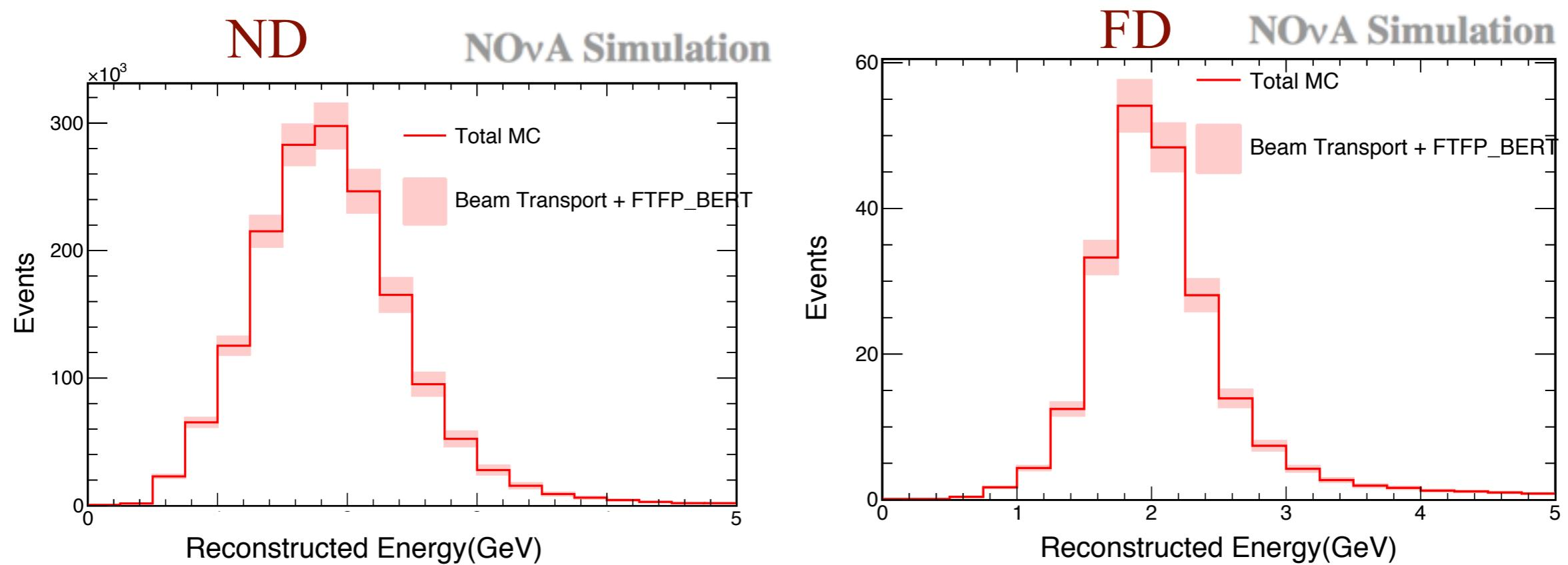
The error band represents a  $\pm 1$  sigma shift of all beam systematics: Hadro-production model(different MC based physics list FTFP\_BERT), Spot size, Beam position on the target (X/Y), Target position, Horn current, Horn-positions, & the modeling of horn's B-field.
