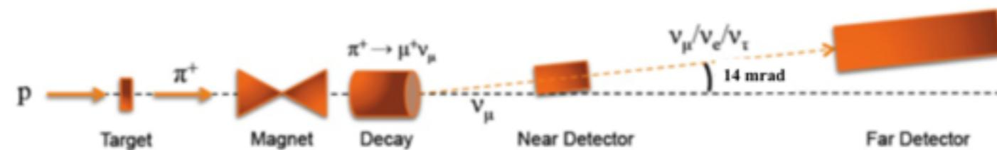
At 14 mrad off-axis, narrow band beam peaked at  $E_\nu=2\text{GeV}$
