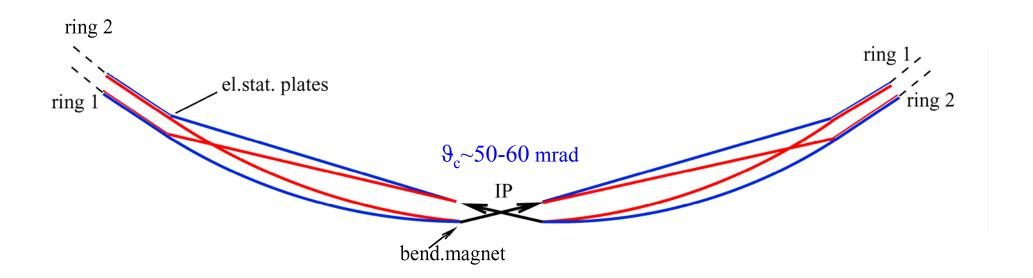
Crab-waist collisions assume collisions at some horizontal angle, that requires 2 rings with electrostatic separators near IP and inside rings, plus one rings for injection, 3 rings in total.
