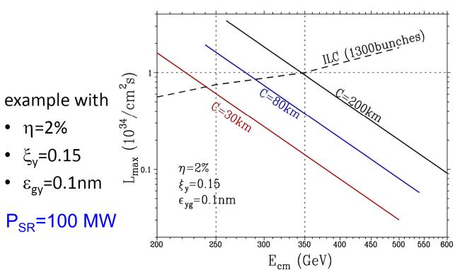
For 2E=240 GeV the luminosities (per one IP) of ring and linear colliders are comparable. But large ring colliders with 4 IP can provide by one order higher luminosity.
