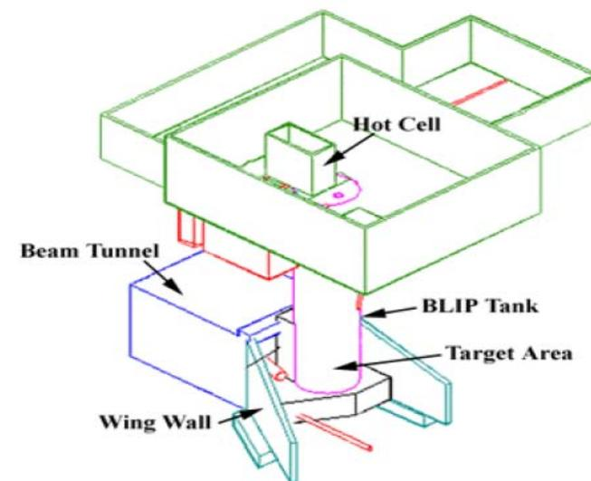
Figure 3. BLIP Beam Tunnel and Target Schematic
