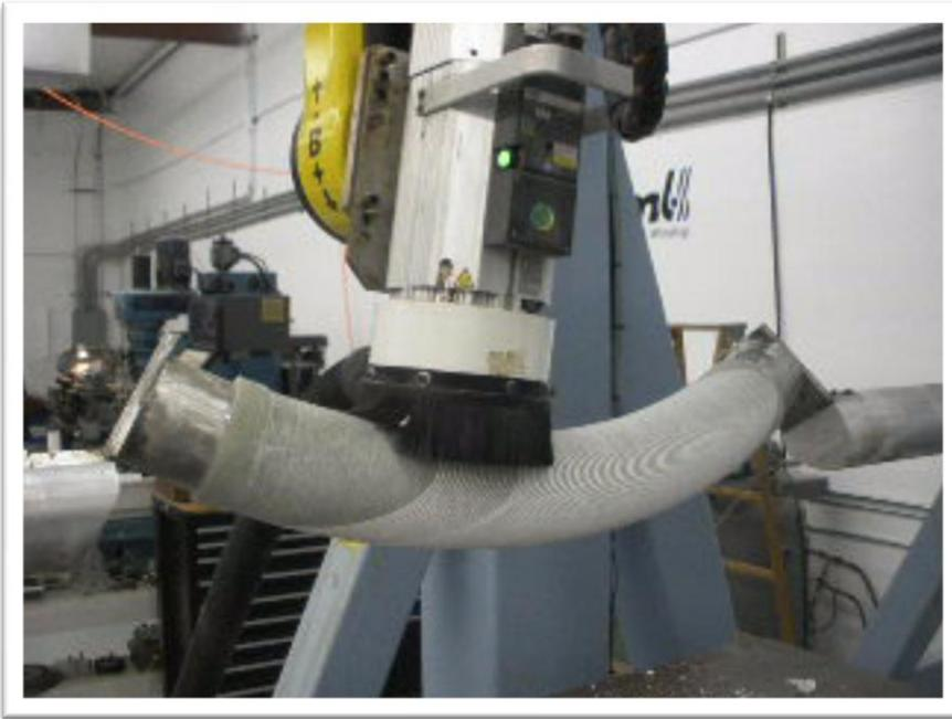
Manufacturing of Bent Coil
