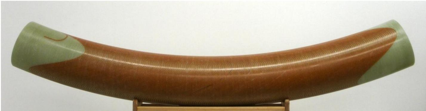
**Combined function magnet – quadrupole with superimposed dipole**
