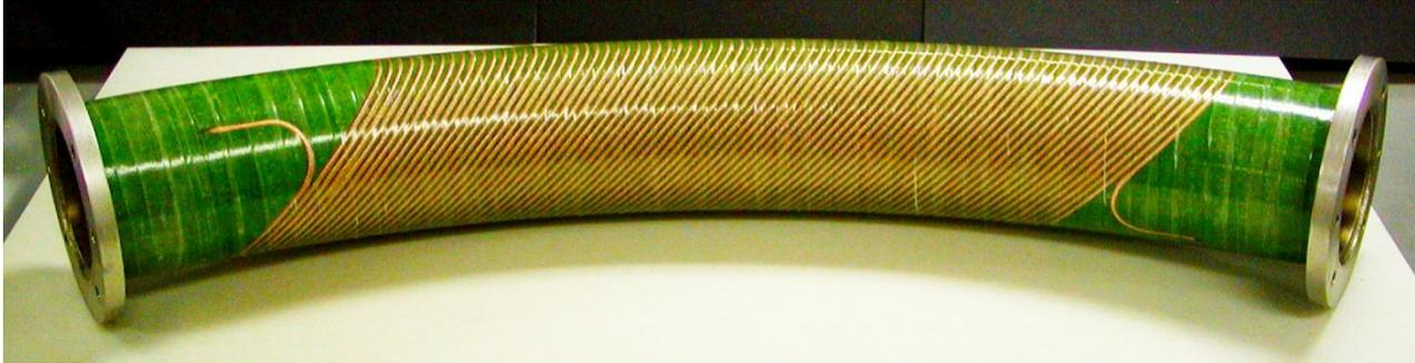
**Bent dipole magnet with compensated quadrupole**
