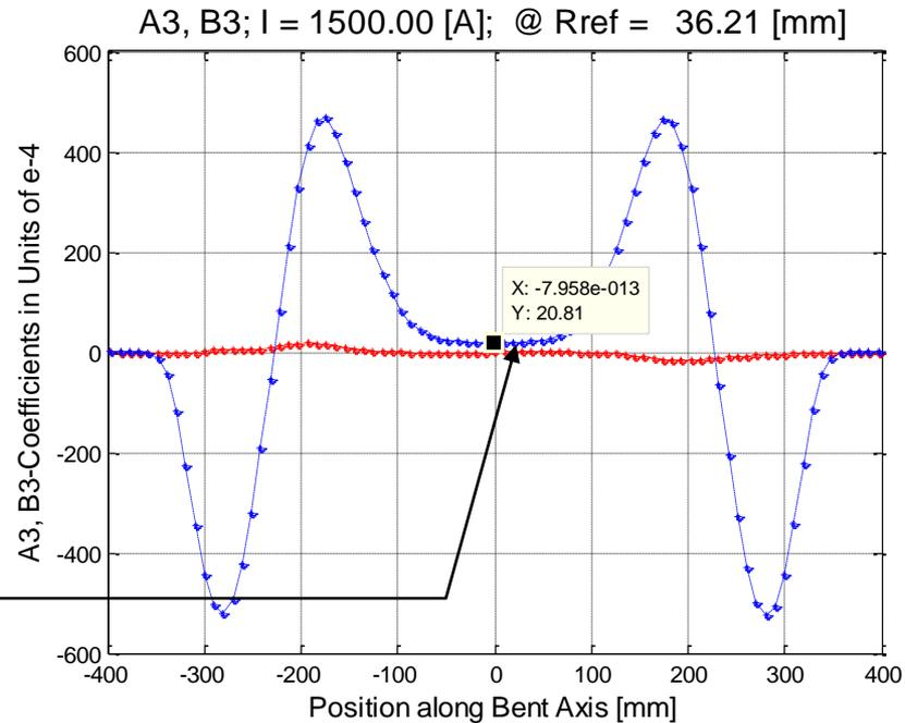
Test coil to qualify coil cross-section of bent dipole
