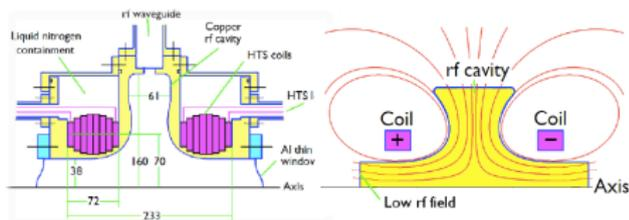
Loss of x 2 gradient advantage in pillbox geometry
