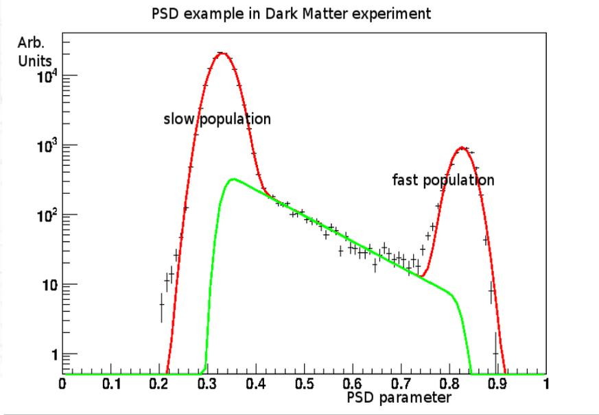
Example of signal/background separation in WArP R&D exp
