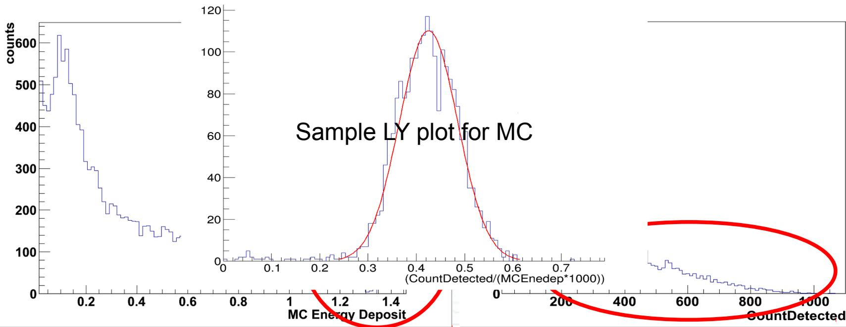
Two Cobalt gamma peaks, clearly visible in MC Energy deposition, smeared in collected photon number
