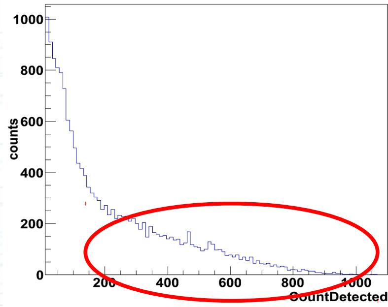
Two Cobalt gamma peaks, clearly visible in MC Energy deposition, smeared in collected photon number
