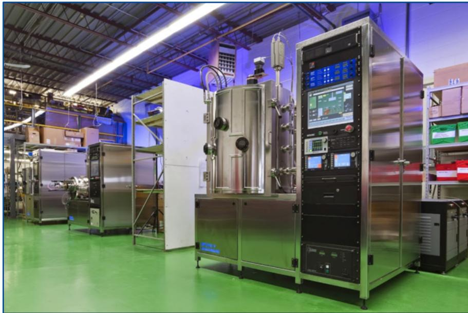
TPB coating (wavelength shifter) of PMTs at INTLVAC in Canada
