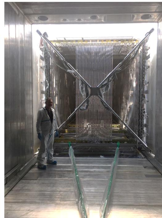
Pulling the 2<sup>nd</sup> T300 into its cryostat – March 29
