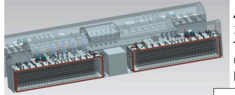
4 identical cryostats W, H, D, 15.1m x 14.0m x 62m
