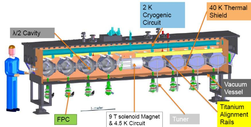
FRIB HWRs and  $\beta=0.53$ HWR cryomodule (courtesy of MSU-NSCL)
