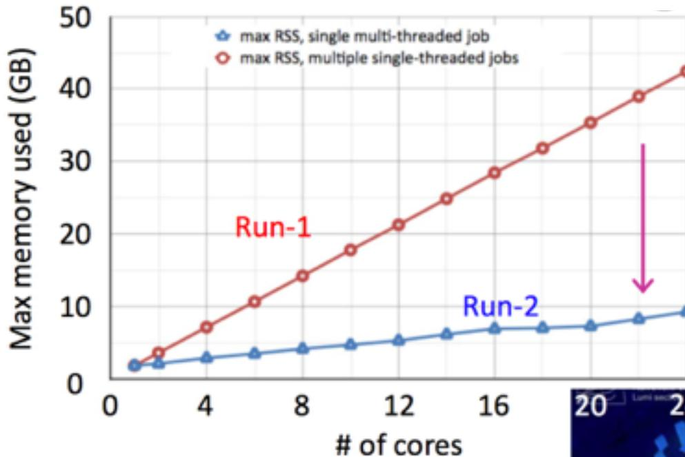
Updating to a multi-threaded framework reduces memory footprint needed to reconstruct events
