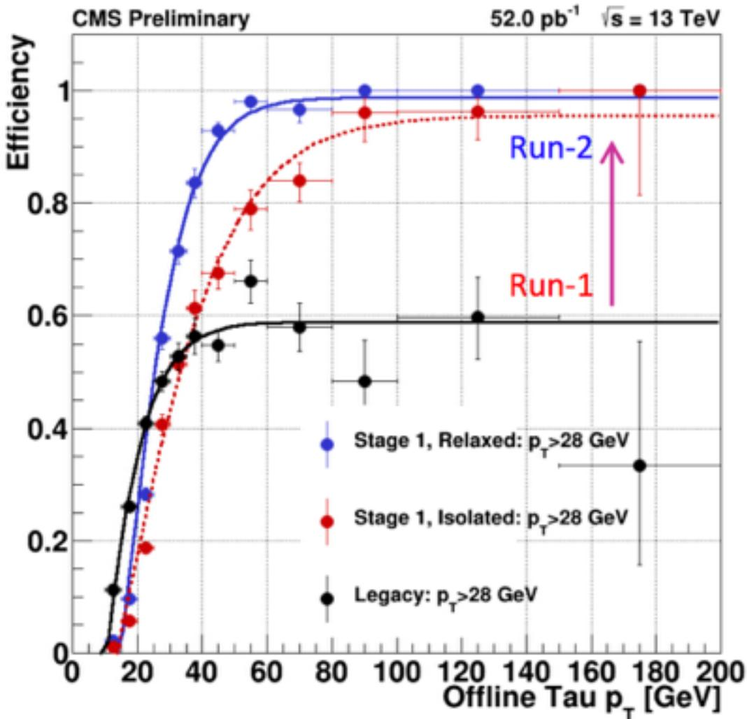
First stage of the CMS calorimeter trigger upgrade in use for 97% of the 2015 run
