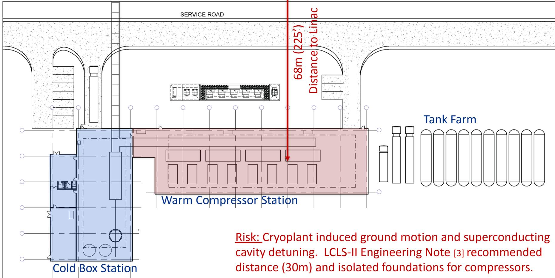
**Risk:** Cryoplant induced ground motion and superconducting cavity detuning. LCLS-II Engineering Note [3] recommended distance (30m) and isolated foundations for compressors.
