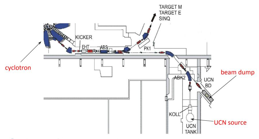
Neutrons are produced in a canneloni-style target (lead inside Zircaloy tubes, 21 cm diameter and 55 cm long), and are then thermalized in an ambient-temperature heavy-water moderator
