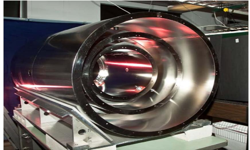
$\mu$ -shields: Shielding factor =  $2 \times 10^4$
