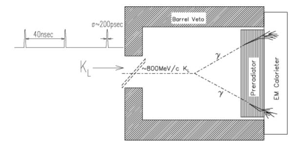
**Figure 9:** Illustration of the key elements of the KOPIO technique: TOF measurement of the K<sub>L</sub> momentum, measurement of  $(\pi^0 \rightarrow \gamma \gamma)$  and veto of all other background process particles.
