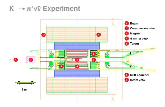
**Figure 7**: Conceptual design of a Project X  $K^+ \rightarrow \pi^+ \nu \overline{\nu}$  experiment based on evolution of BNL E949.
