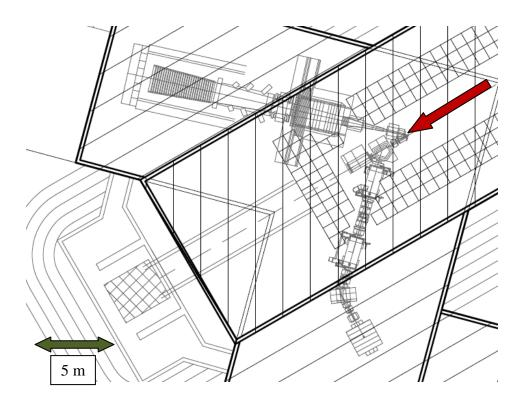
**Figure 5**: The NKX (above) and the CKX (below) concept beamlines and experiments served with a common production target (3 GeV proton beam indicated with red arrow).
