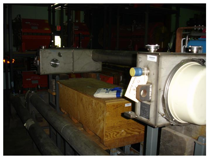
The spool piece provides the cryo and power connection between the 2 strings of magnets while providing an open drift space in between. One of several existing optical tables can be placed Meren Chou, FCPA retreat 2010
