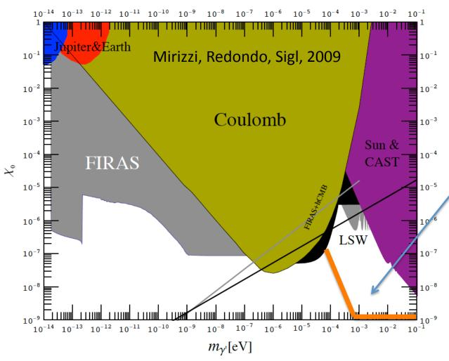
For a cavity-enhanced resonant regeneration experiment, F=10<sup>5</sup> gives a factor of 300 improvement previous LSW experiments.
