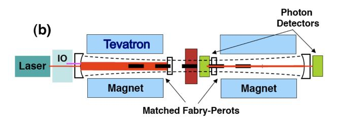
Matched Fabry-Perot cavities shape the axion beam and resonantly enhance the axion-photon transition probability. Light leaks coherently from the bright cavity into the dark cavity.
