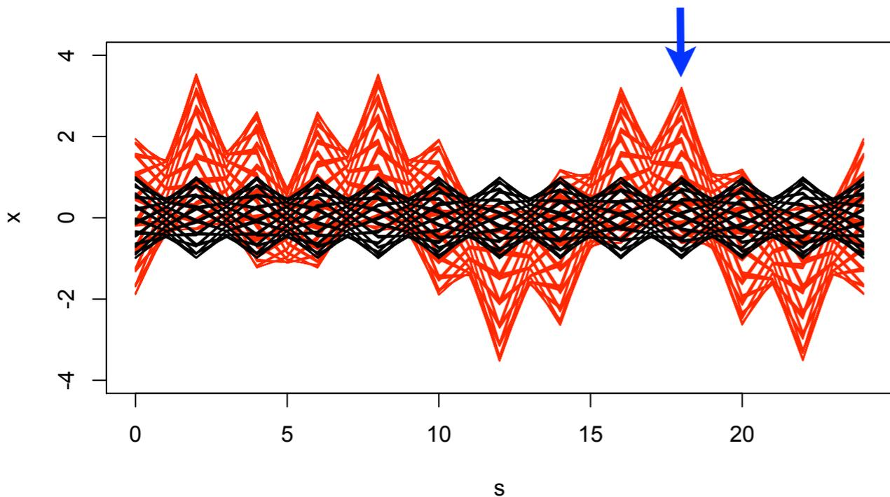
Orbit distortion due to single dipole field error
