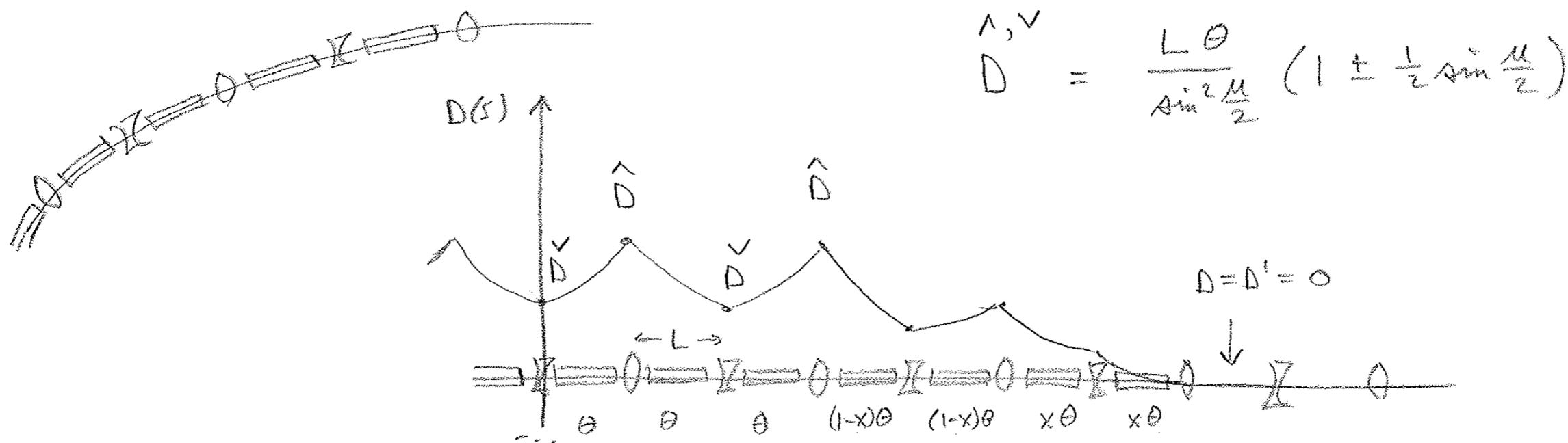
So, dispersion of a periodic FODO lattice w/ bending can be
